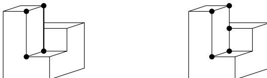
The bold line shows an edge shared by three faces; by adding a vertex on that line we create an extra edge so that every edge is shared by exactly two faces.
