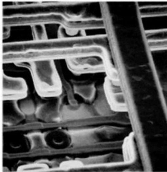
Figure 1.2 Image of an integrated circuit with different layers, form Lucent Technologies.
