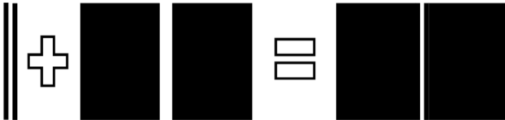
Figure 5.1: Patterns exposed on high and low voltage, where overlapping of two structures leads to the final electrode structure electrodes.
