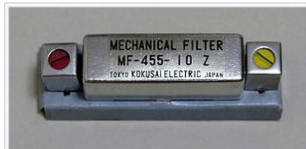
Figure 1. A mechanical filter made by the Kokusai Electric Company intended for selecting the narrow 2 kHz bandwidth signals in SSB radio receivers. It operates at 455 kHz, a common IF for these receivers, and is dimensioned 45×15×15 mm ( 1\frac{3}{4}\times\frac{7}{12}\times\frac{7}{12} in).
