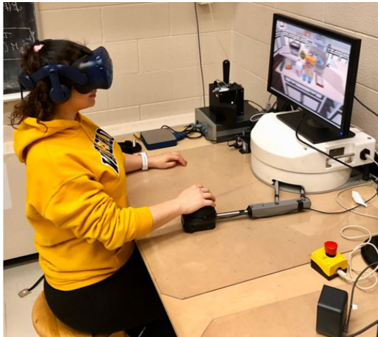
(a) Manipulandom upper-limb rehabilitation robot (end-effector based robot) used in this research
