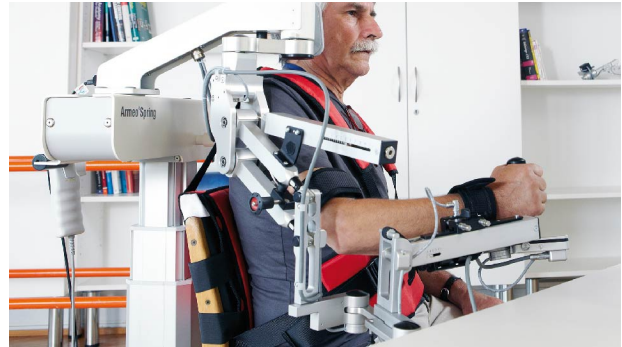
(b) Armeo Spring (exoskeleton robot), reproduced with the permission from [16]
