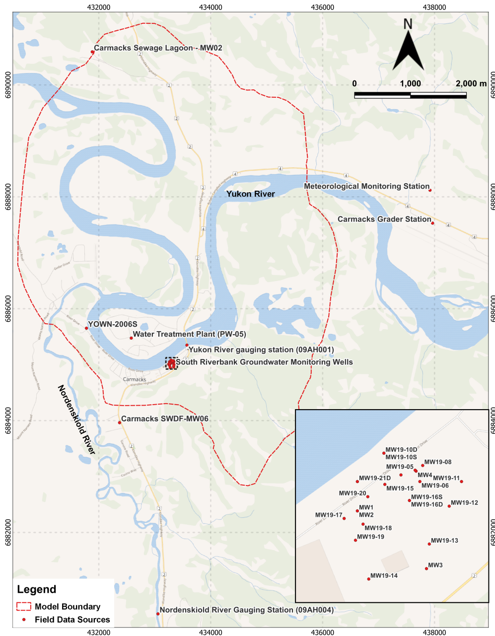
Figure 9. A plan view map shows the locations of field data collection points. The inset map demonstrates the detailed information on the South Riverbank Groundwater Monitoring Wells in the dashed black box. The collected data from these collection points were used to assign model properties and boundary conditions and used for model calibration. Background map data: © OpenStreetMap (2023).
