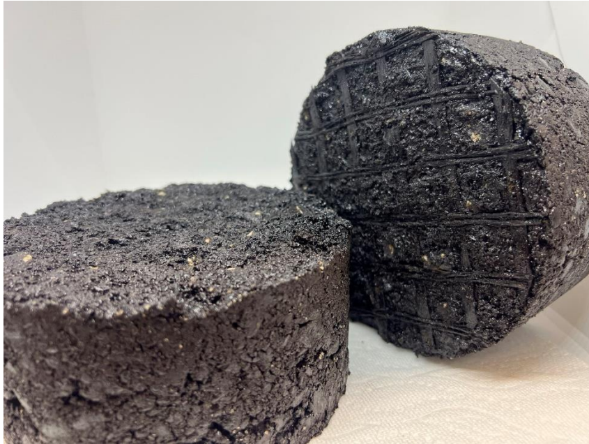
Figure 6-6 Sample Separated After Standardized Freeze-Thaw Conditioning
