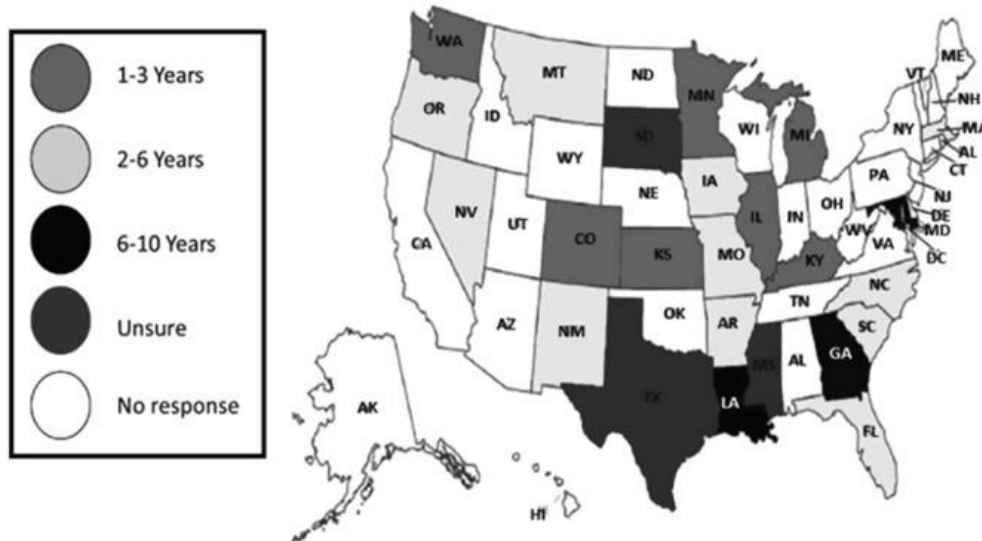
Figure 2-1 Average Service Life of A 40–50 mm Asphalt Overlay in the United States (Kwon et al., 2005)
