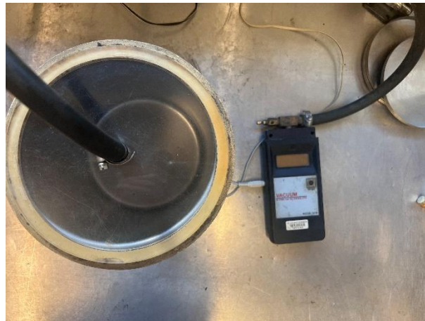
Figure 3-10 Maximum Relative Density Test
