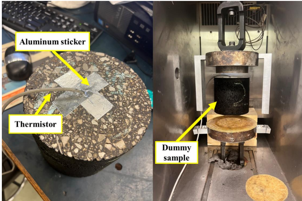
Figure 6-2 Dummy Sample in the Chamber Monitoring Temperature
