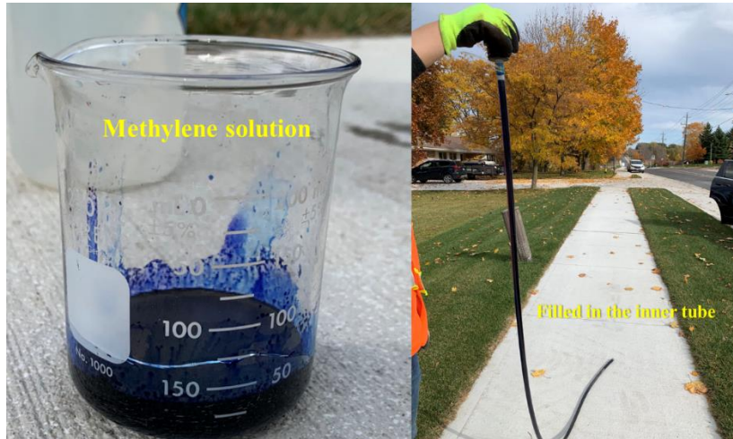
Figure 4-15 Methylene Solution Filled in Frost Tube
