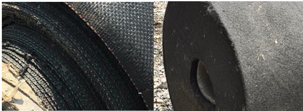
Figure 2-5: Geotextile Products: a) Woven; b) Non-Woven (Titan Environmental Containment, n.d.)
