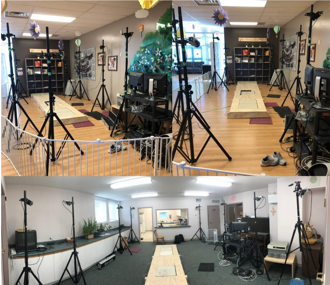
Figure 4.1: The walking platform and camera locations in the two early learning centres.
