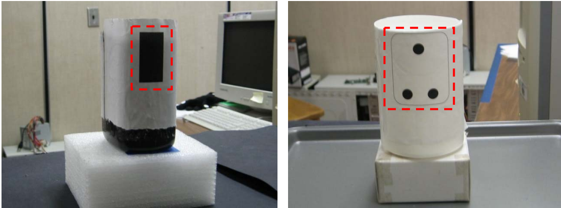
Figure 4-9: Patterns attached to the bottle (left) and cup (right). The black rectangle and the three black markers were used to identify the bottle and cup, respectively.
