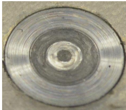
Figure 33: Weld surface of refill friction stir spot weld of Al 6063/DP 600 under the condition of 1800rpm, 2s of dwell time, 1.1mm of plunge depth, 1.5s of retract time
