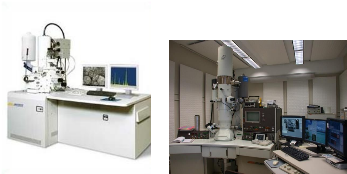
Figure 28: JEOL JSM-6460 equipped with Oxford Instruments INCA-350 energy-dispersive spectroscopy system (left) and JEOL 2010 TEM/STEM is a field emission Transmission Electron Microscope (right) [40]
