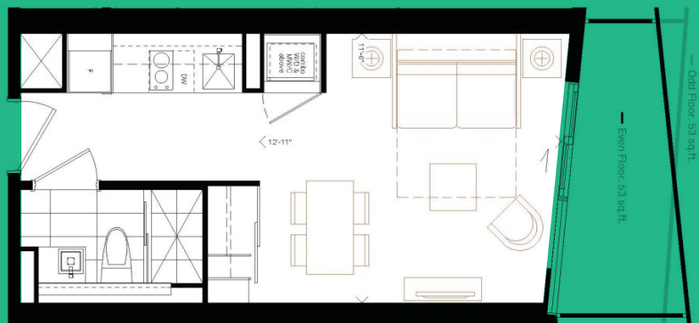
FIGURE 50 Smart House Toronto Unit Plan This unit prioritizes spatial efficiency. It combines the sleeping and entertaining area. The kitchen is incorporated into the entry corridor.
