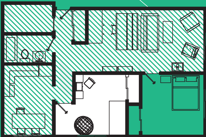
FIGURE 48 Basement Apartment Plan A standard 2-bedroom apartment in a 3 storey walk-up. This unit has a large amount of shared space.
