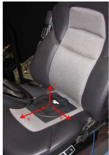
Figure 13: Here is a picture of the rubber seat pad that you will be sitting on. The rubber can bend and conform to your buttocks.
