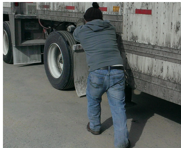
Figure 4. A) Dollies are buried in the snow during the winter season, making it a challenge for drivers to pull out of the snow; B) The driver has to lift, pull and push the dolly to hook up the trailers; C) The driver also has to lift, pull, and push a lever to release the landing gear of the trailers.
