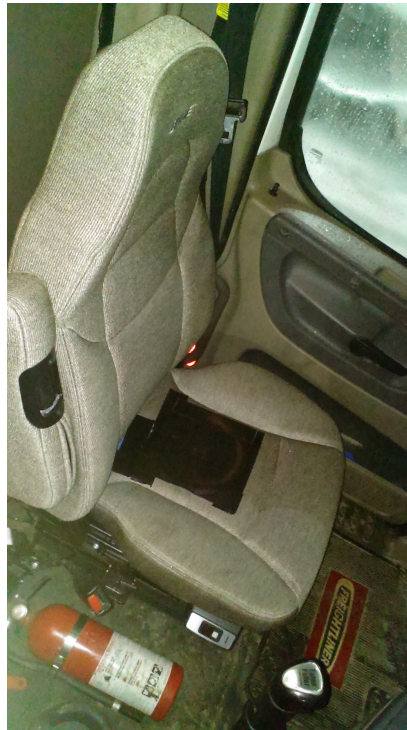
Figure 8. Set-up of the accelerometer and seat pan secured onto the truck seat.
