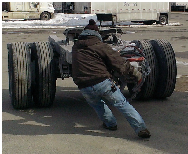
Figure 4. A) Dollies are buried in the snow during the winter season, making it a challenge for drivers to pull out of the snow; B) The driver has to lift, pull and push the dolly to hook up the trailers; C) The driver also has to lift, pull, and push a lever to release the landing gear of the trailers.
