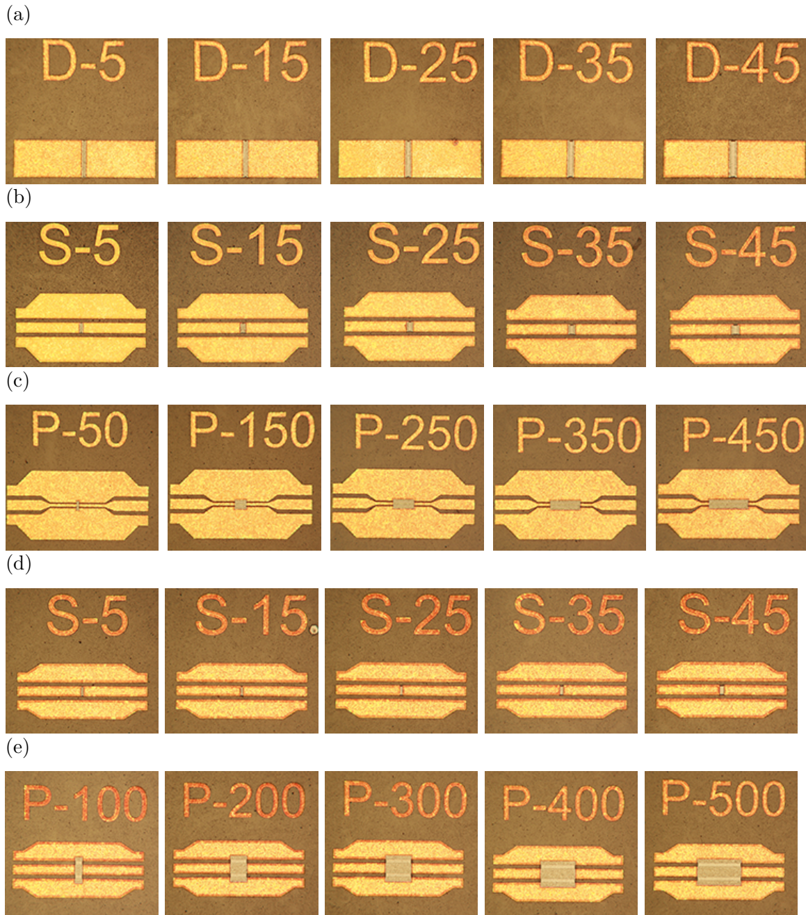
Figure 3.7: Fabricated devices included in the mask layout for this project. The number above the device defines the size of the gap or the width of the short in \mu\text{m} . (a) DC switches with variable gaps (b) CPW series switches ver1, with variable gaps (c) CPW parallel switches ver1, with variable shorts (d) CPW series switches ver2, with variable gaps (e) CPW parallel switches ver2, with variable shorts.
