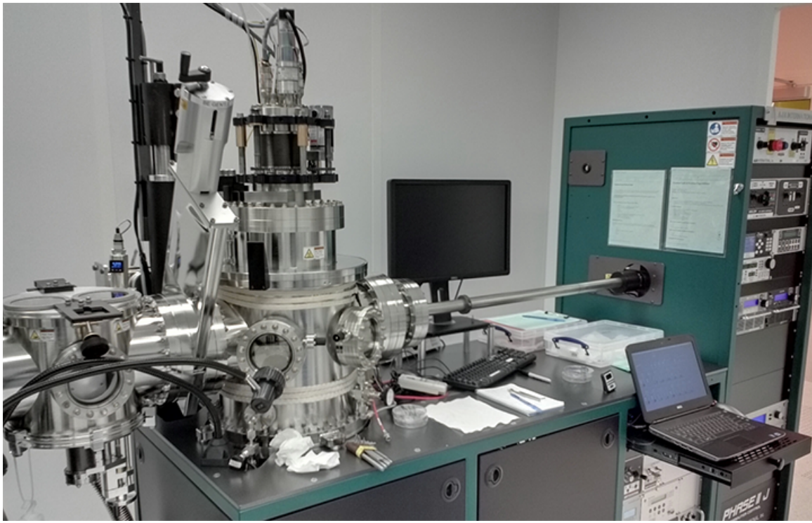
(a) Metals deposition chamber of the twin chamber AJA ATC Orion Series sputtering system
