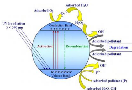
Fig. 5.3: Photoexcitation of a semiconductor (taken from ref. 118 with permission from Elsevier).
