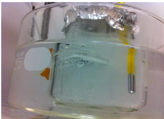
Fig. 5.6: Hydrothermal growth of ZnO nanorods.
