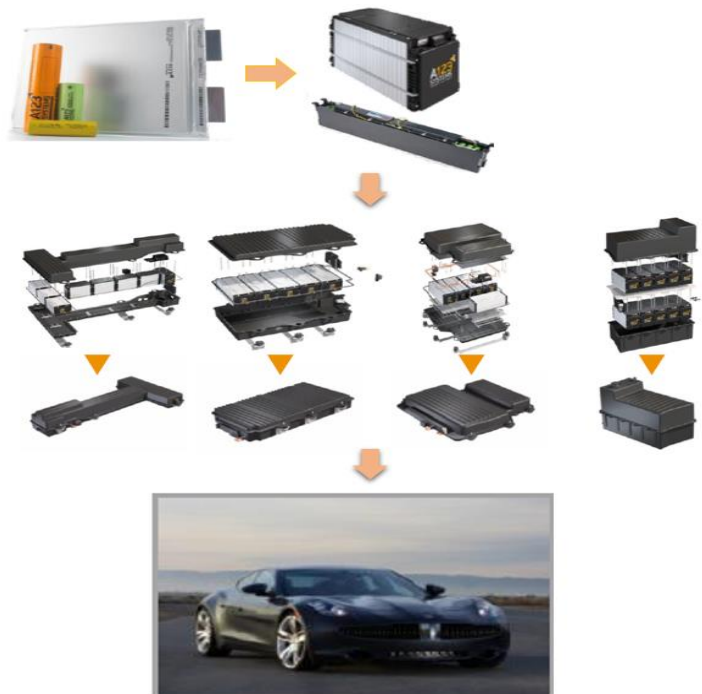
Figure 18: Battery pack system constructions: cells-modules-packs [34].
