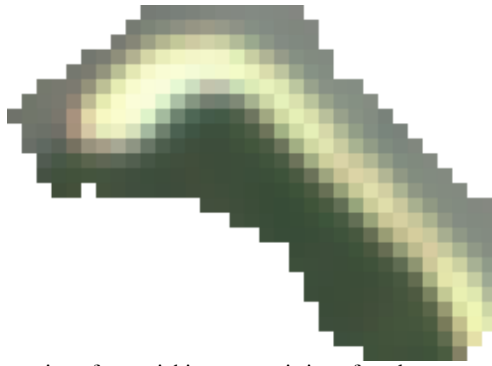
Figure 3.3.1 A portion of an aerial image consisting of road pavement (top), sidewalk (middle) and grass (bottom).
