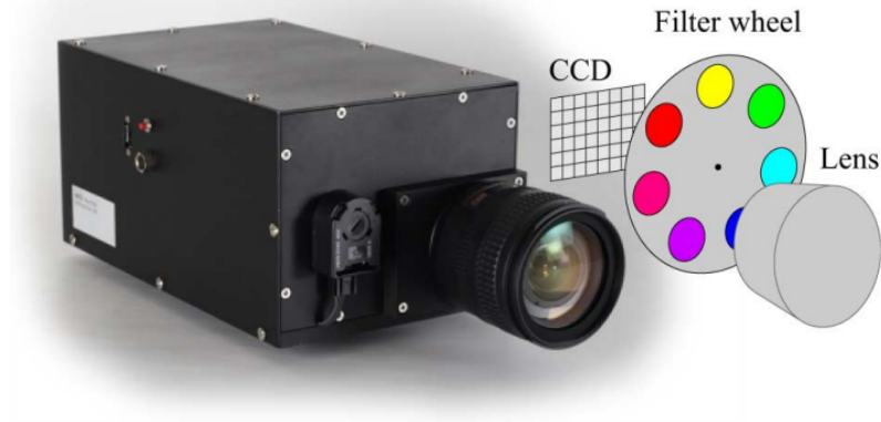
Figure 2.2: A example of a filter wheel with seven optical bandpass filters for sequential multispectral imaging [18].
