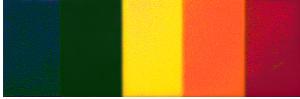
Figure 4.3: The test icon used in the second set of experiments. The true reflectance spectrum was measured for each unique section of the icon and then compared to the predicted spectra from the three inverse methods. These inverse methods are the state-of-the-art Wiener estimation method (WEM) and the proposed Wiener-based demultiplexer (DEMUX-WEM) and random forest-based demultiplexer (DEMUX-RFM).
