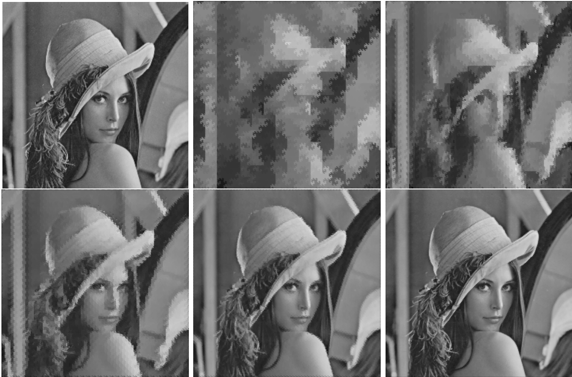
Figure 3.7: Fractal-wavelet (LIFSW) coding with base (-1 + i, \{0, 1\}) : The original 512 \times 512 image of Lena is in the top lefthand corner. The other images, from top to bottom, left to right, result from choosing the domain level to be -13 , with ranges -11, -9, -7, -5, -3 .
