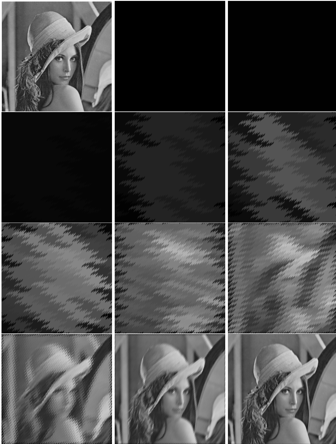
Figure 3.2: Pruning with base (-2 + i, \{0, 1, 2, 3, 4\}) : The original 512 \times 512 image of Lena is in the top lefthand corner. The other images, from top to bottom, left to right, result from pruning the wavelet trees at levels -11 to -1 .
