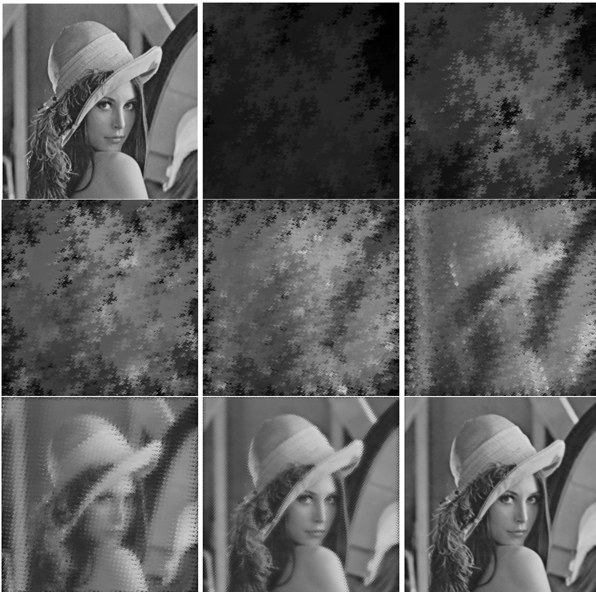
Figure 3.9: Fractal-wavelet (LIFSW) coding with base (2 + i, \{0, 1, i, -i, -2 - 3i\}) : The original 512 \times 512 image of Lena is in the top lefthand corner. The other images, from top to bottom, left to right, result from choosing the domain level to be -9 , with ranges taking all values between -8 and -1 .
