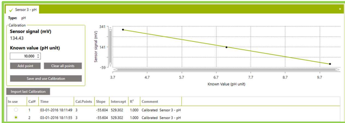
Figure D-6. Calibration curve for pH microelectrode.
