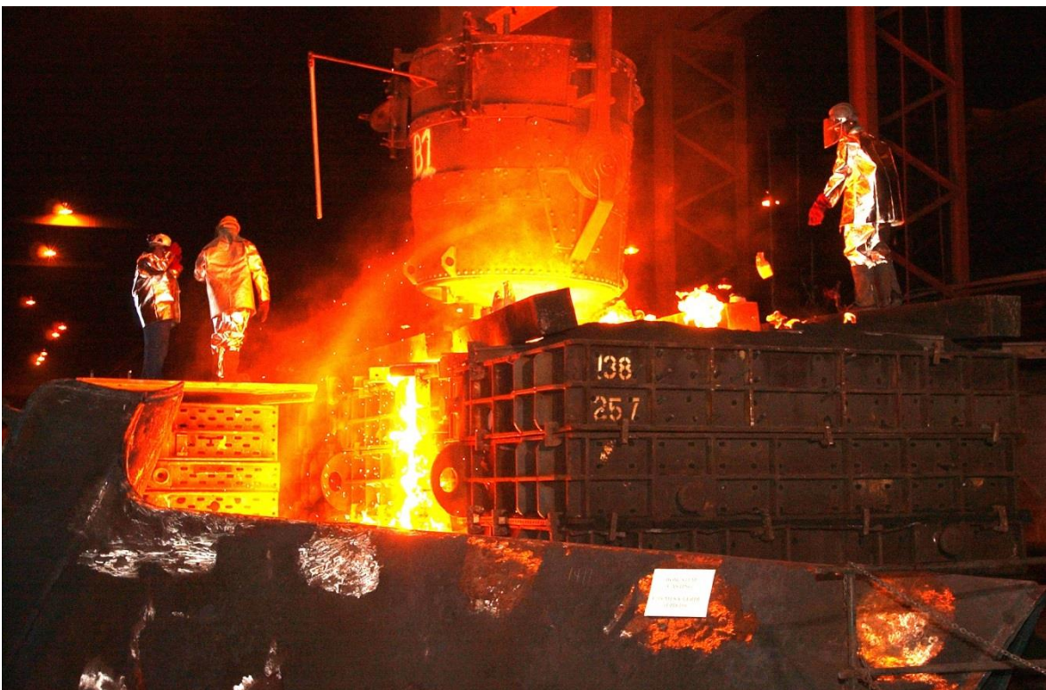
Figure 5-3: Electric arc furnace for steel production
