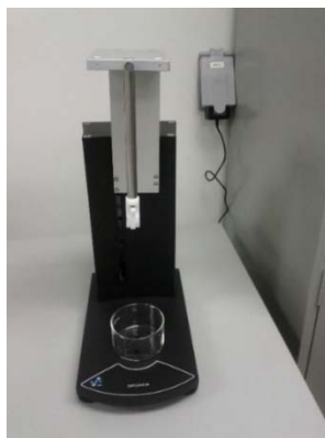
Figure 2.10: Image of automatic system for dip-coating in CAPDS lab.
