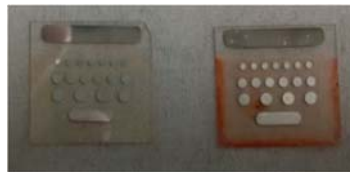
Figure 9.3: Image of fabricated planar CdSe QD-heterojunction solar cells. There are 18 cells with different active area (metal pad area) on the samples.
