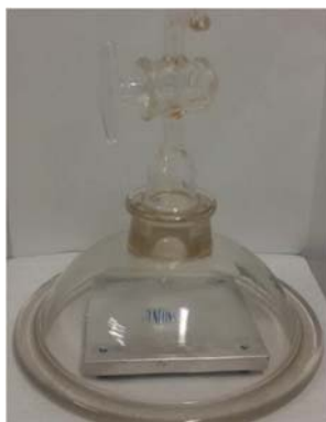
Figure 5.1: Set-up (leveled stage inside desiccator) used for drop-casting deposition of quantum dots.
