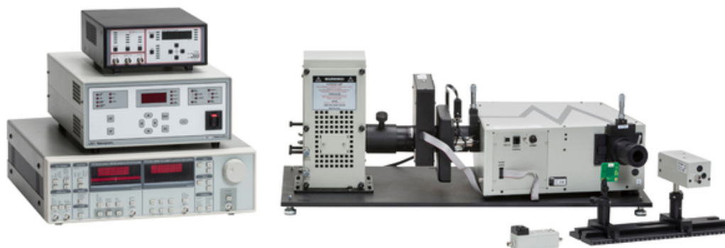
Figure 3.14: Photograph of EQE measurement system components.
