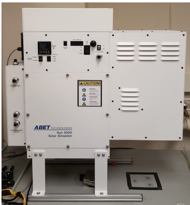
Figure 3.11: Photograph of solar simulator from ABET Technologies.
