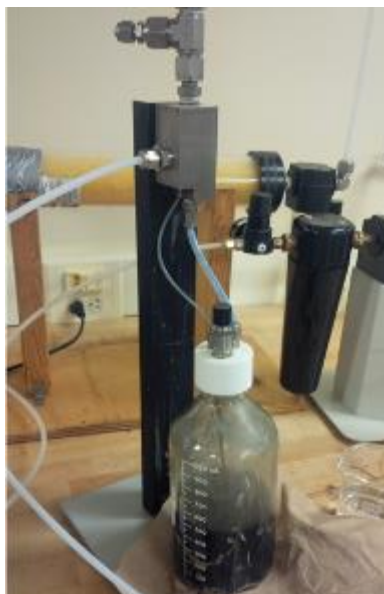
Fig. 20 TSI atomizer subsystem, aerosolizing an iron nanocolloid
