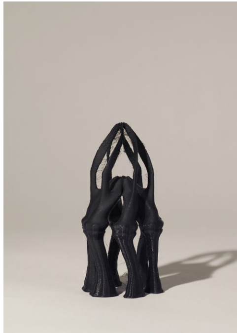
fig 2.09 sculptural figure #1 Using the array tool in Modo, a single bone-like column was modeled, polar arrayed and joined at the top. An improper printer setting resulted in the formation of webs of plastic between the six thin pieces joining at the top.
