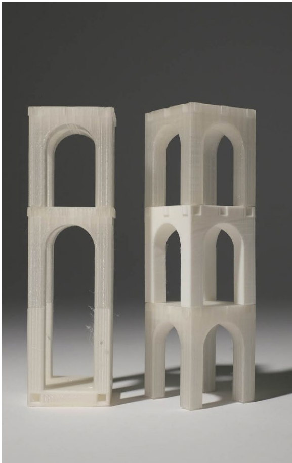
fig 2.13 modular toy Inspired by Lego, these are modular arch toy blocks with interlocking pegs. After each printing, the interlocking mechanism is modified for better performance.
