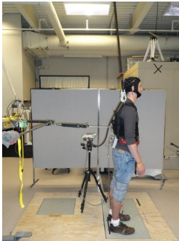
Figure 3.1: Experimental set up: Lean and release system to evoke perturbations. Perturbations to standing balance were achieved using a custom-made lean and release cable system that reliably
