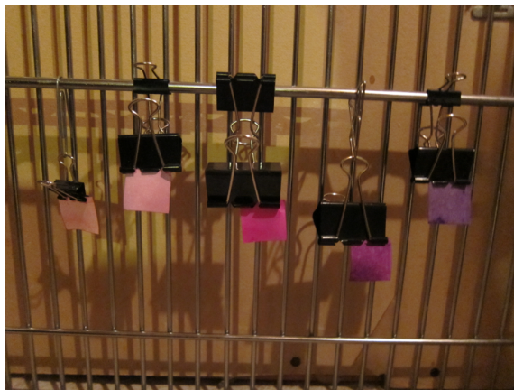
Figure 7.4: Paper samples soaked in pigment or in dye solutions are hung to dry in order to ensure that the colourant does not settle toward one face of the paper.
