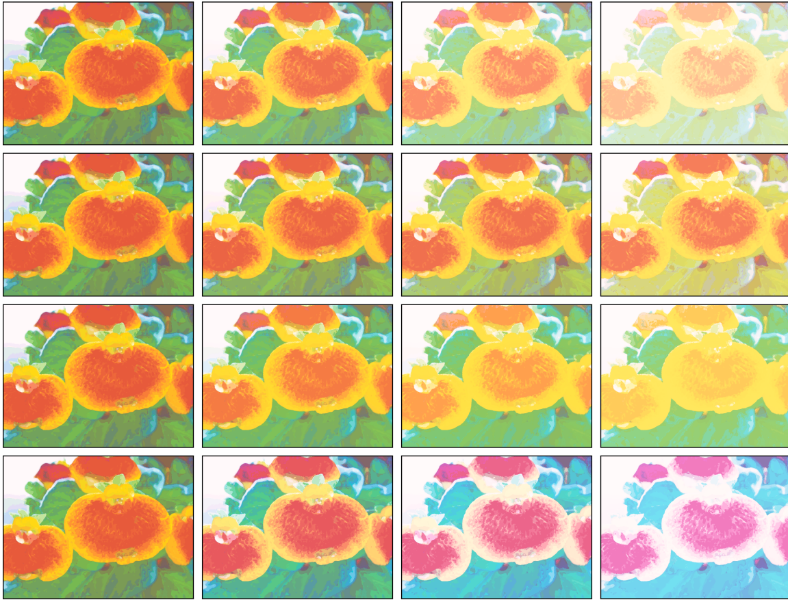
Figure 8.7: Rendering of an image composed of mixtures of cyan, magenta, and yellow pigments is faded according to four hypothetical sets of fading rates for a total exposure of 4.365 \times 10^7 \text{ J m}^{-2} . The sets of fading rates used are indicated in Table 8.4. Top Row : The pigments fade at perceptually similar rates. Second Row : The cyan pigment fades more rapidly. Third Row : The magenta pigment fades more rapidly. Bottom Row : The yellow pigment fades more rapidly.
