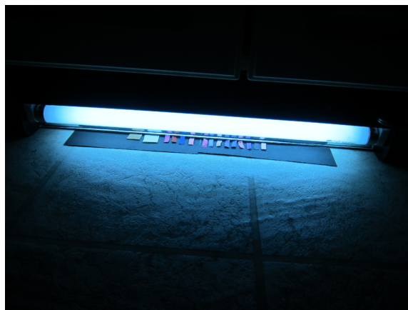
Figure 7.10: The emission from a fluorescent lamp may vary across the length of the bulb. Here, the bulb is dimmer at the ends of the tube.
