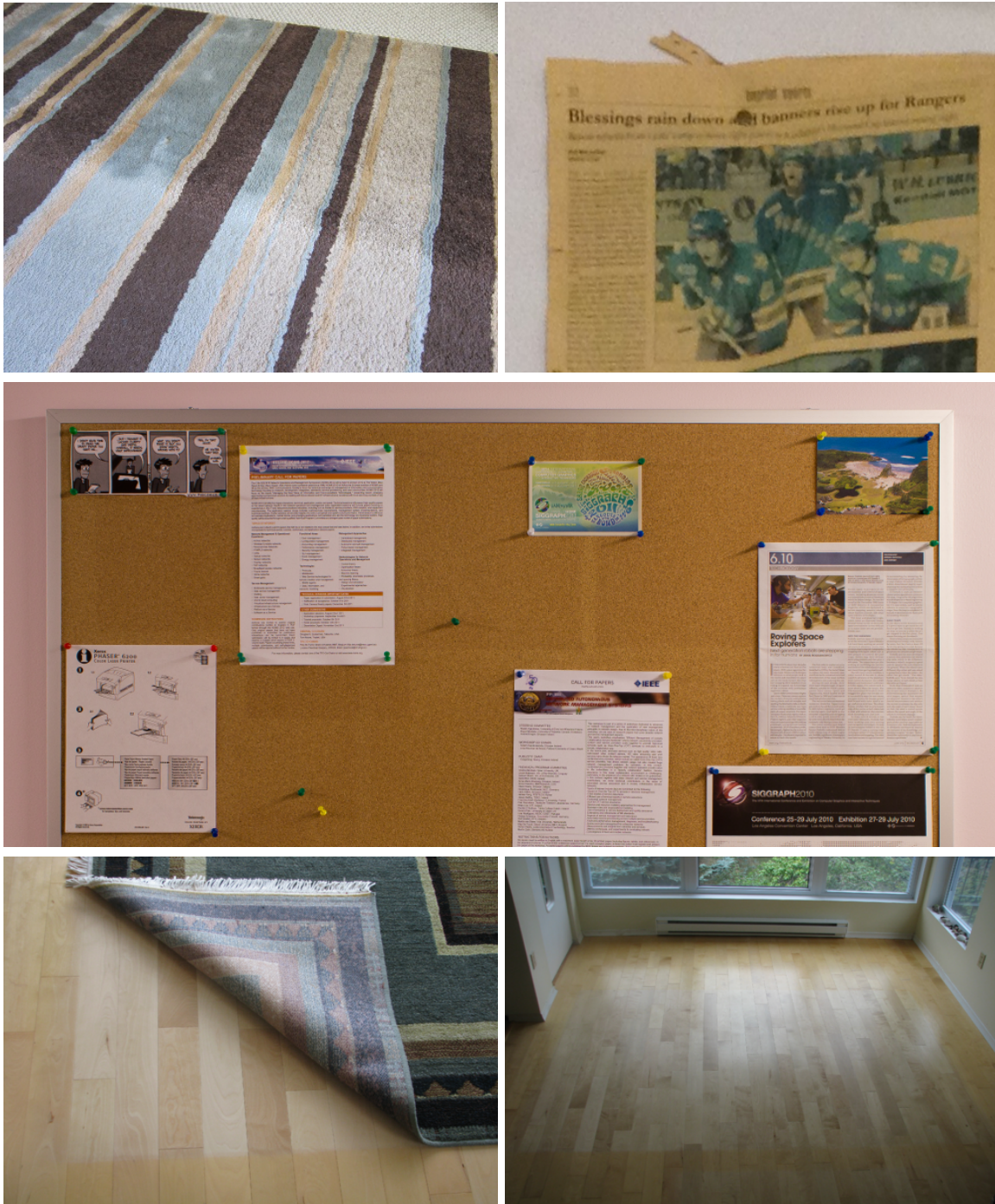
Figure 1.1: Photographs depicting common materials subjected to fading due to light exposure. Top Left: An area rug has faded everywhere except where a couch had been placed. Top Right: A newspaper has turned yellow from many years of light exposure. Middle: Printed materials have been added and removed from a bulletin board over time, resulting in an irregular fading pattern. Bottom: Wood flooring darkened from light exposure except where covered by a rug.
