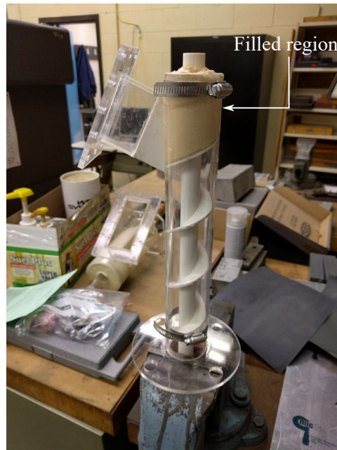
Figure 3.3: The swirl injector with the unused section filled in with the epoxy-filler mixture.
