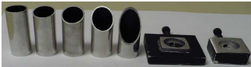
Figure 5: A set of fixed sample holders, transmission and reflection port adapters
