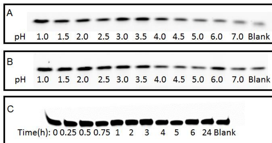
Figure 4.5 Gel electrophoresis micrographs showing the stability of (A) A 15 and (B) a random DNA (DNA 26) incubated at different pH values for 1 h, and (C) A 15 incubated at pH 3.0 for various amount of time.
