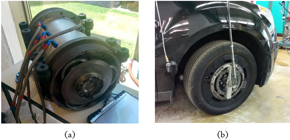
Figure 4.4: (a) Electric motors (b) wheel hub sensors for force/moment measurement.
