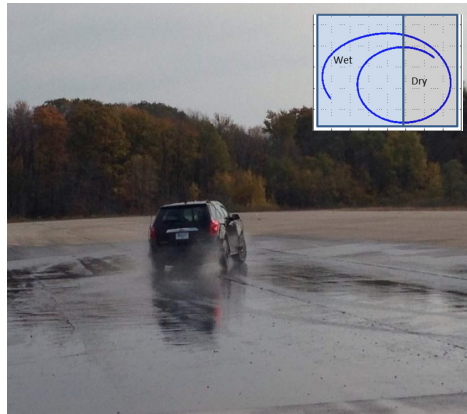
Figure 5.35: AWD vehicle in full turns on dry/wet sealer
