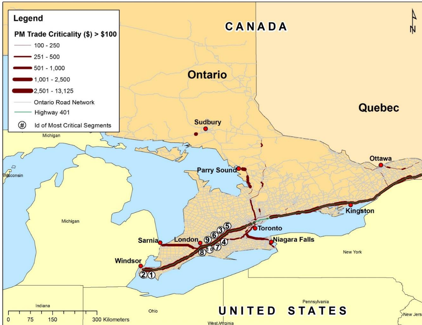
Figure 6-2- Trade criticality of Ontario’s highway infrastructure during the PM peak. IDs of most critical segments are listed in Table 6-2
