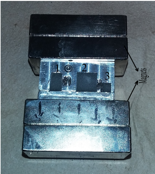
(a) Three different Terfenol-D sample sizes in mold.
