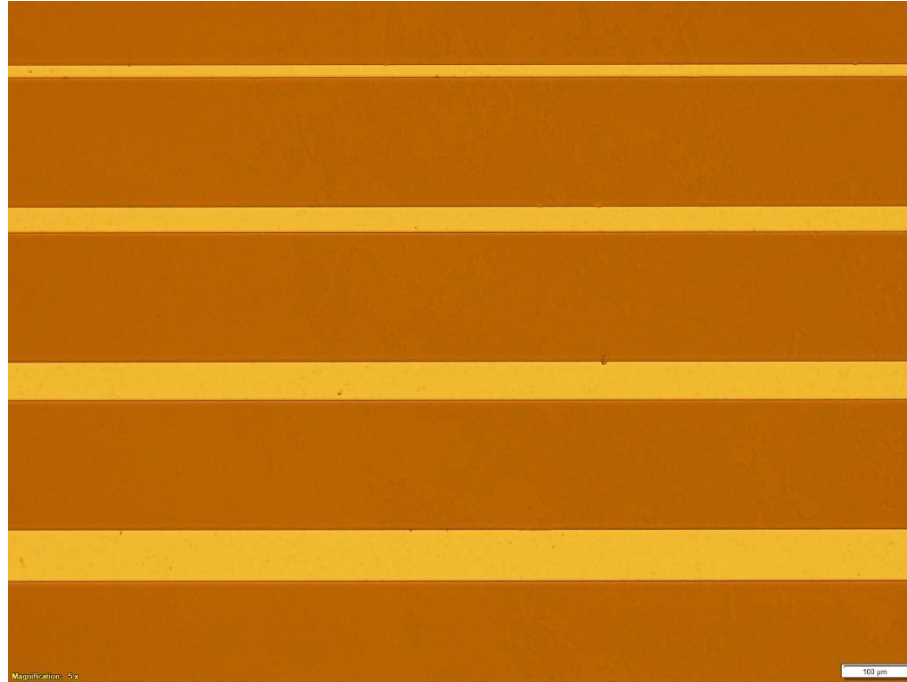
Figure 5.3 Microscopic view of the gold pattern, which becomes the top metal layer after the lift-off process. The widths of the 4 mesa ridges are 80, 60, 40, and 20 \mu\text{m} from bottom to top in the figure.
