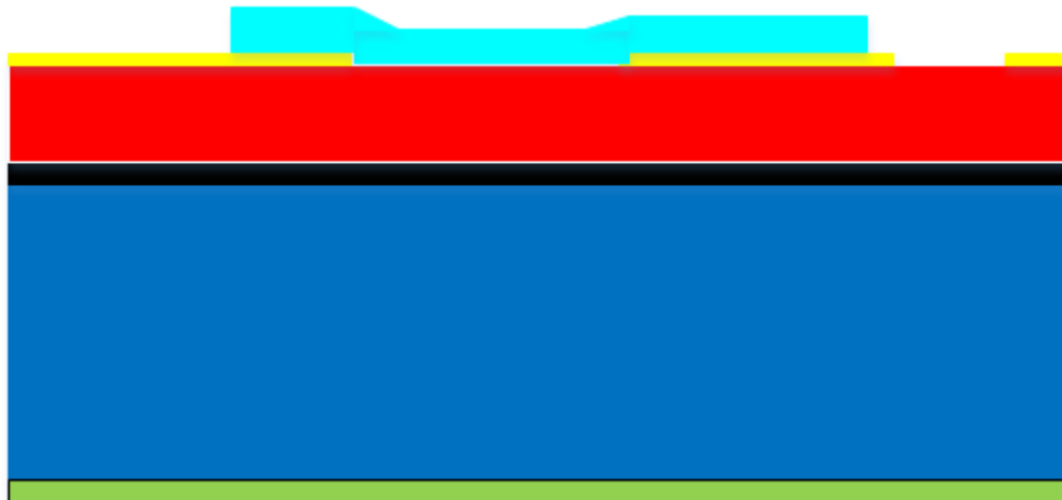
Figure 3.4 Piezoelectric material is deposited by reactive sputtering and patterned using positive photoresist and the second mask, PZFILM
