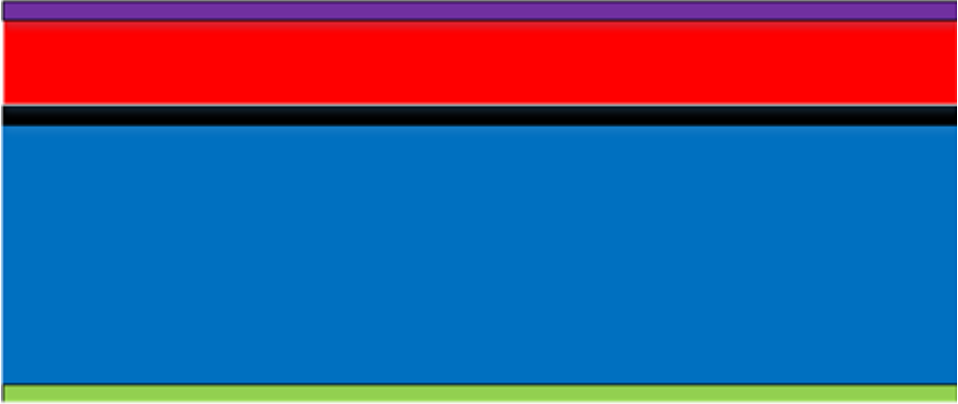
Figure 3.2 PSG (purple) deposited on SOI, which is also protected by bottom oxide
