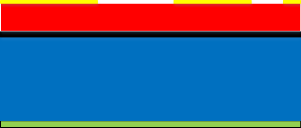
Figure 3.3 Thermal oxide is grown and patterned by the first mask, PADOXIDE
