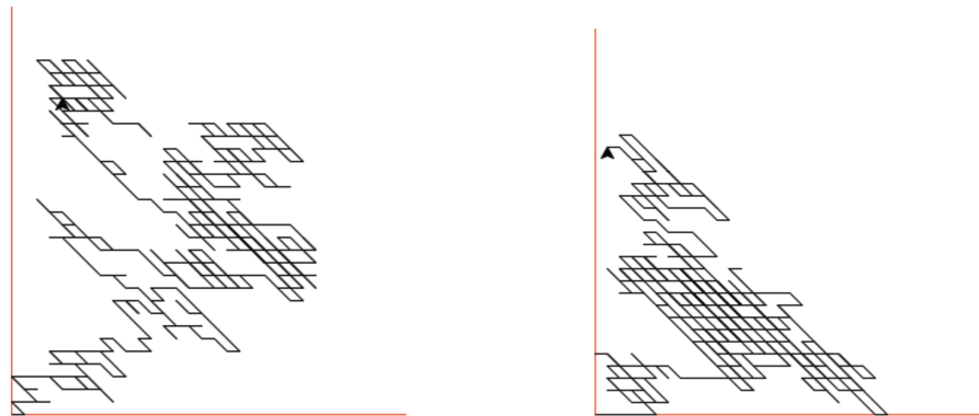
Figure 11.3: Two uniformly sampled Gouyou-Beauchamps walks on 800 steps: an unweighted (balanced) model (left) and a weighted (reluctant) model with parameters a = \frac{1}{\sqrt{2}} and b = 1 (right), which can be scaled to a model with step weights of 1 and 2 by uniformly multiplying each weight by \sqrt{2} .
