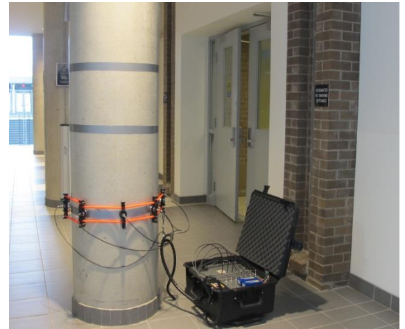
Figure A-4: Column STC2 tested in Science Teaching Complex (4700\sqrt{f'_c}) [1]
