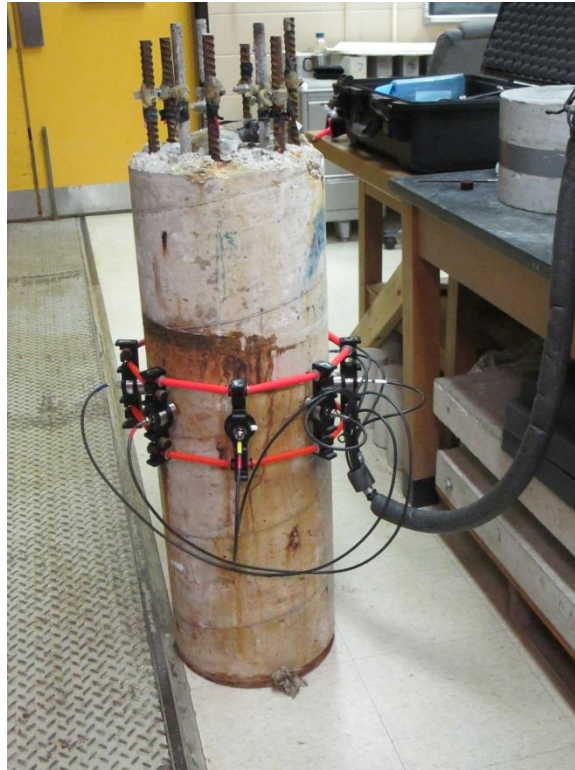
Figure 7-18: Damaged column tested in the laboratory
