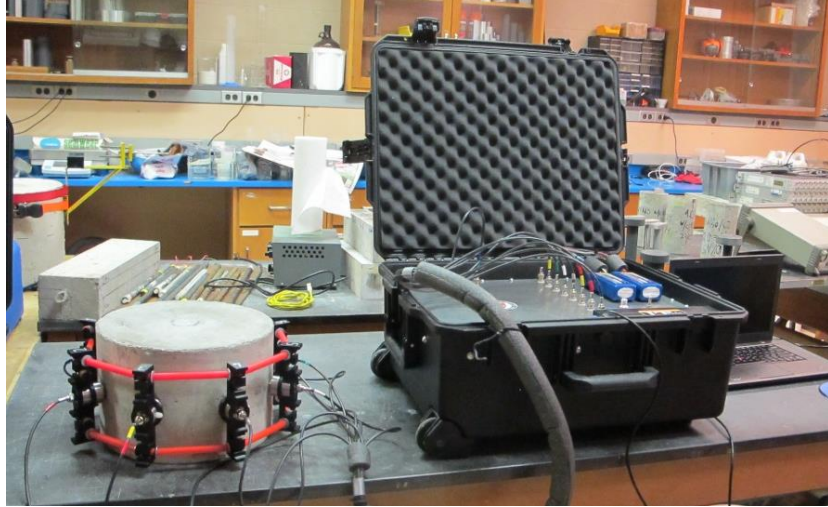
Figure 7-1: Setup for the verification of the equipment and testing of the coupling system proposed
