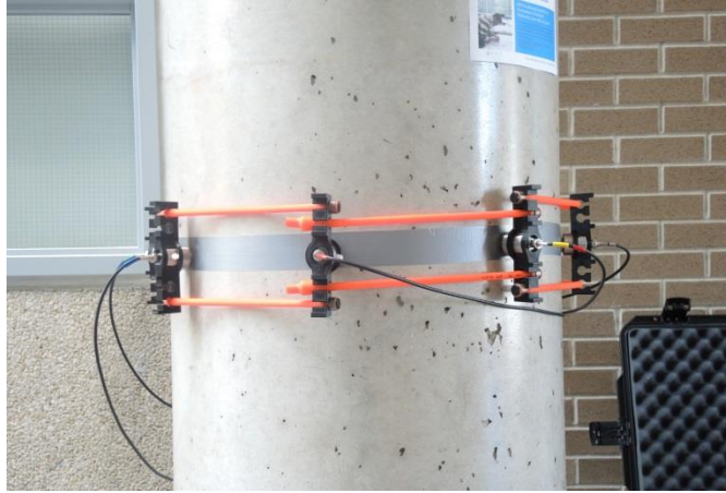
Figure 3-7: Final design of the adjustable sensors array
