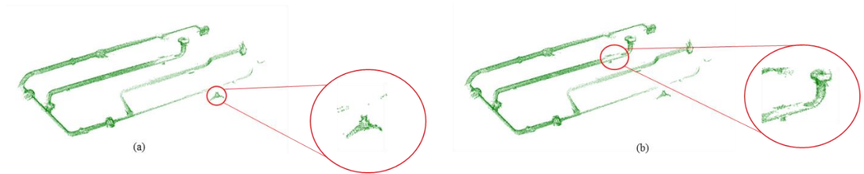
Figure 5-5. Challenges of removing clutter points without removing points on the object of interest.
