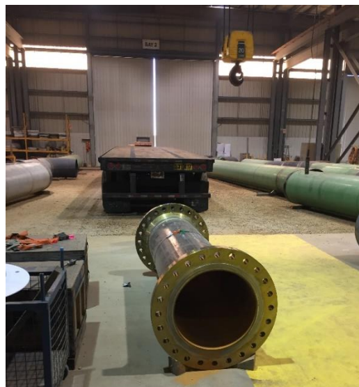
Figure 2-17. Spool ready to be shipped out.
