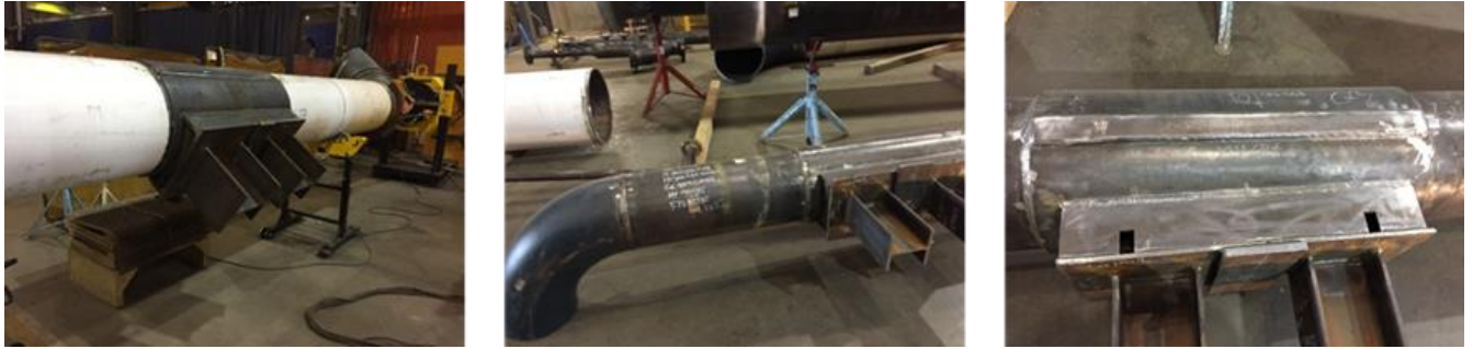
Figure 2-2. Structural component, generally referred to as shoe.
