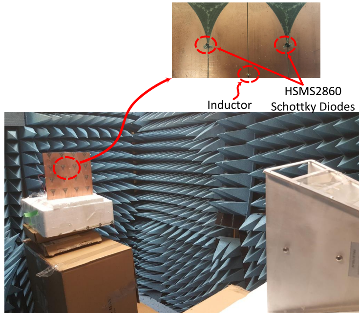
Figure 6.10: The experimental setup showing the transmitting antenna and the TCA surface in an anechoic chamber. The inset shows the position of both the series inductor and the Schottky diode.
