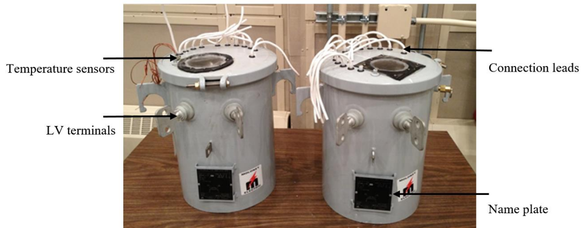
Figure 3-1: Photograph showing model transformers T1 and T2.
