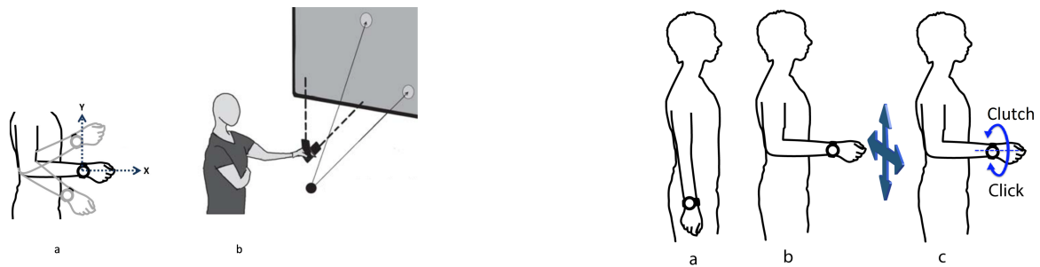
Figure 3.1: Left: Pointer manipulation in the rotation techniques, W1RR and P1RR, is governed by the orientation changes of the control device. (a) For W1RR, the user must sweep the entire forearm to cause changes orientation of the smartwatch. (b) For P1RR, the user can use the wrist sweeps as a more subtle form of manipulation; Right: W1RR can calibrate the center frame of reference from inactive state (a) to raising the arm in front (b) to switch to manipulation mode. From this mode, a 45 wrist flick outwards and back can be used to trigger a click action (c).
