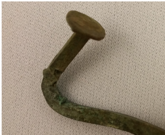
Figure 18. Detail of nail showing cut marks in bend
