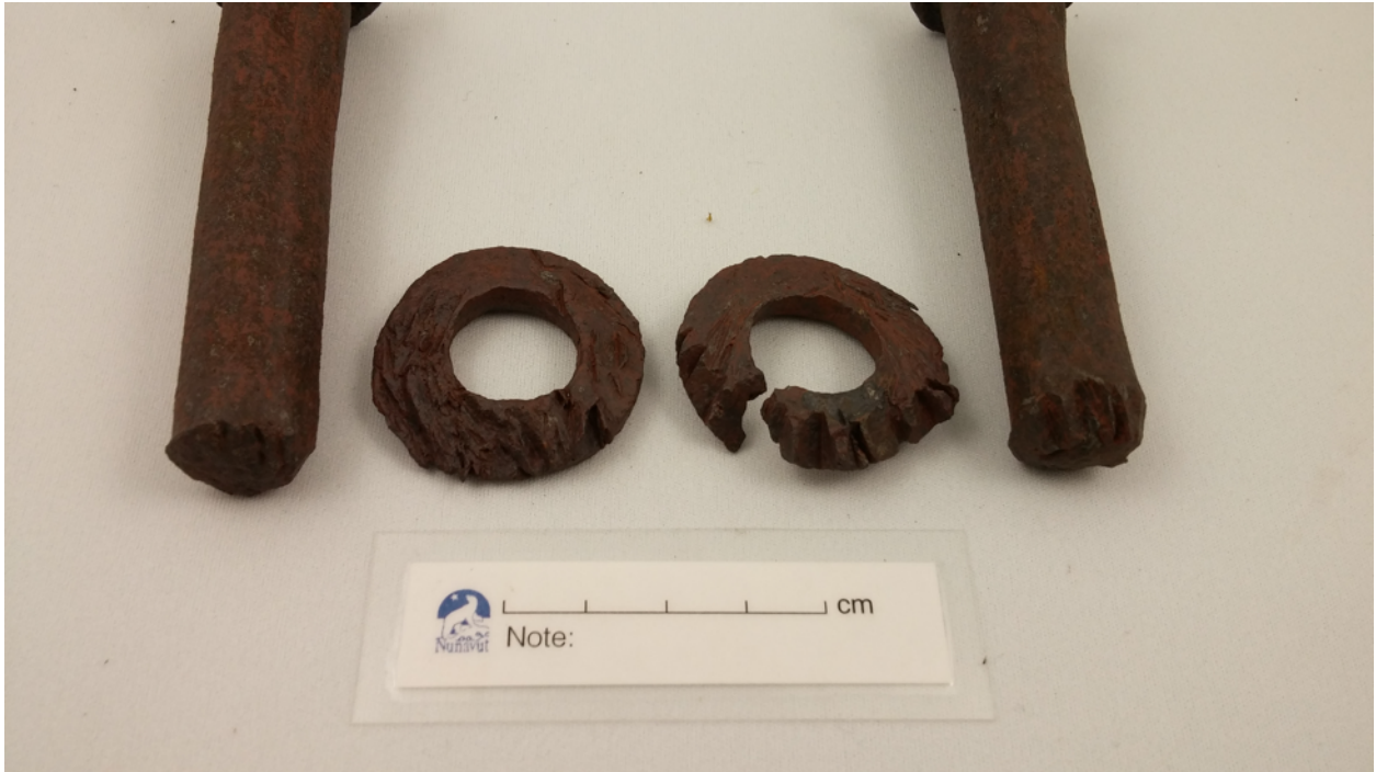
Figure 10. Bolts and clinch rings with chop marks
