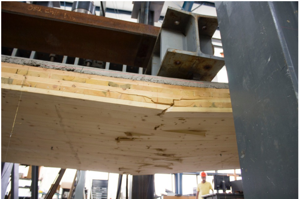
Figure 4. Lumber failure during three-point stress test (Lynch “SOM’s Timber Tower”)
