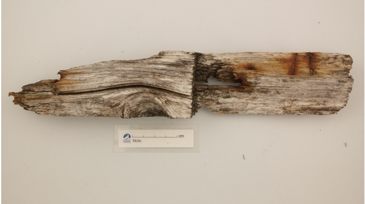
Figure 9. Wood fragment broken up to saw mark with nails removed from broken section
