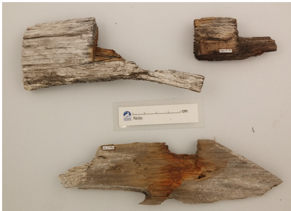
Figure 8. Wood fragments that are broken up to a saw mark
