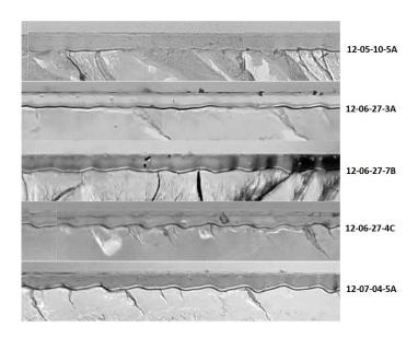
**Figure 7.** Collage showing depths of each of the channels for the chips corresponding to the above electropherograms. The regions shown are the last 3 mm of the separation channel up to 1.5 mm from the BW well but are representative of the separation channel as a whole.
