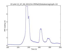
Figure 8. An electropherogram representative of a PCR-CE-based diagnostic, showing primers (near 140 s) and a  $\beta 2M$  product (near 165 s) and an HV1 product (near 175 s), at 236 bp and 345 bp respectively.
