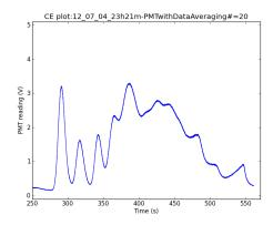
**Figure 5.** An electropherogram from chip 12-06-27-4C, of the size standard (much as above). Only the first 3 peaks are clearly demarcated from their neighbours.
