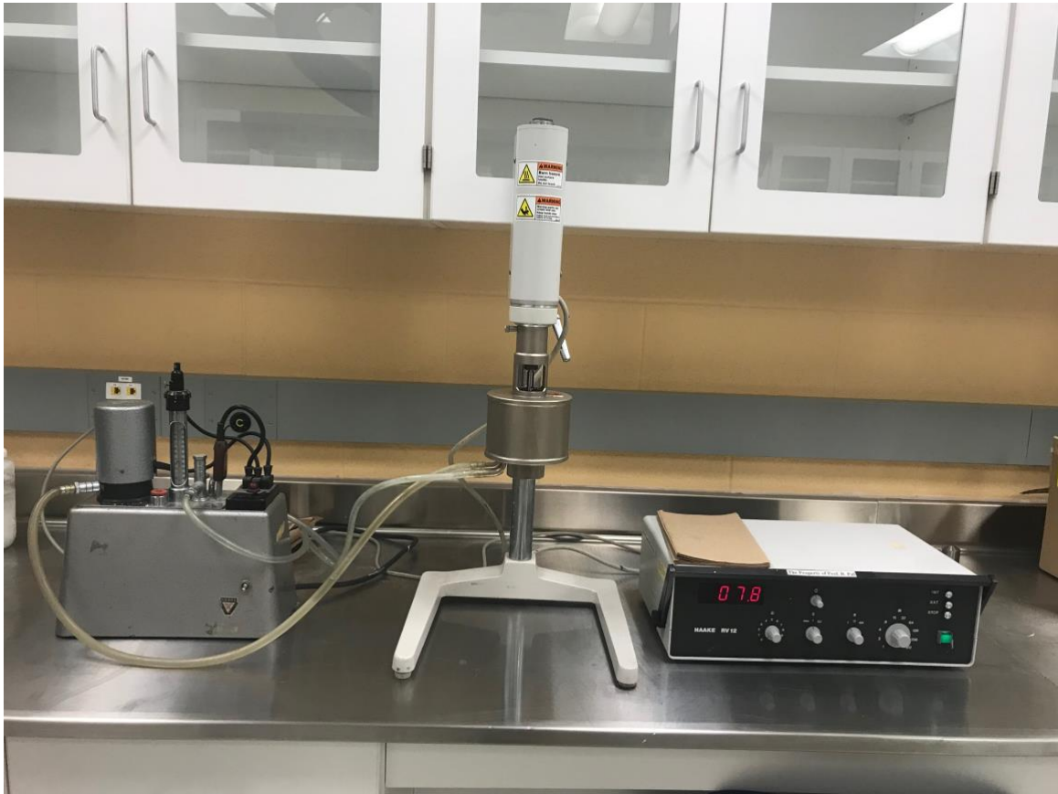
Figure 10: The Haake coaxial viscometer setup.
