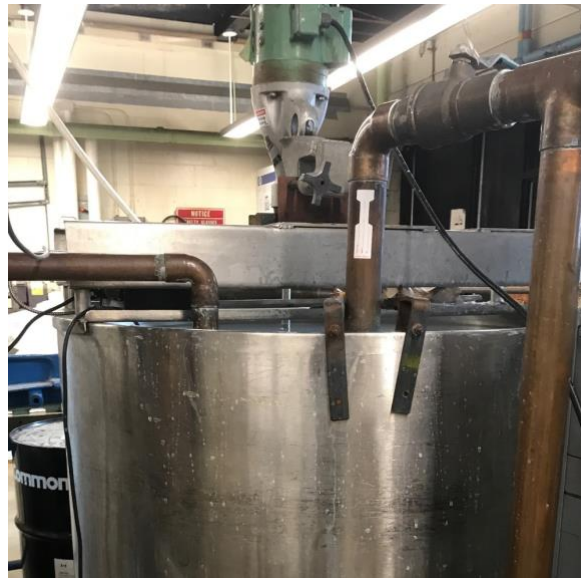
Figure 13: Different sections of the pipeline flow loop system (a) Control panel; (b) Different diameter pipelines; (c) Computer terminal of data acquisition system; (d) Mixing tank
