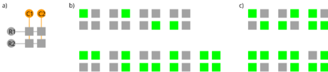
Figure 4.2: The operation of a a) row-column addressed 2 \times 2 array; illustrating the element activation combinations (in green) that are b) allowed; and c) forbidden
