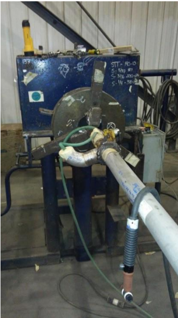
Figure 16: Pipe spool prepared for roll weld
