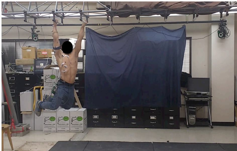
Figure 18: Image of a study participant performing the climbing task on the climbing apparatus. Rungs were affixed to a TRX suspension training system. The participant alternated the support hand for each upcoming rung. The eight rungs used as climbing supports were attached to a TRX.
