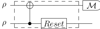
Figure 5.2: Simplified circuit for SPAM tomography method. Repeating the operations in the dashed box m times has the same effect as in the full circuit, Figure 5.1.
