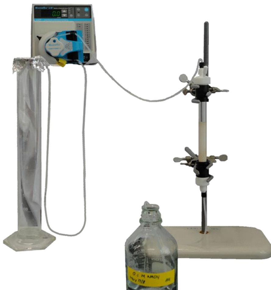
Figure 6: Experimental set up for evaluating DOC hydrophobicity by DAX-8 resin fractionation as per (Song, et al. , 2009)
