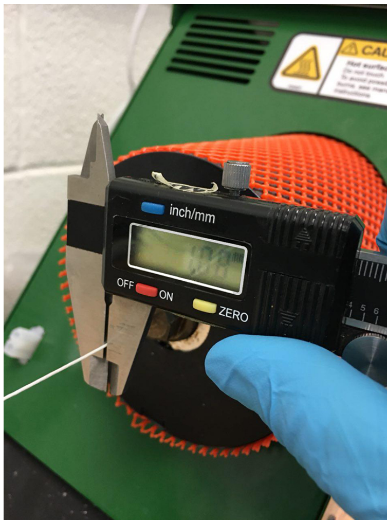
Figure 4.1: Extruded filament- the caliper reads a diameter of 1.08\text{ mm}
