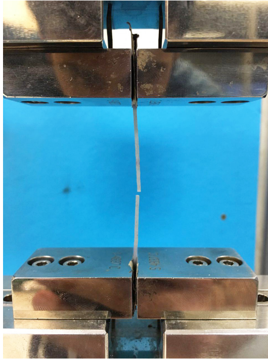
Figure 3.2: A filament held between micro-tensile machine jaws (after failure)
