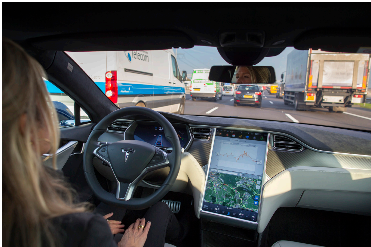
Figure 3.2 - Tesla's autopilot systems are classified as Level 2 and require constant user control at all times
