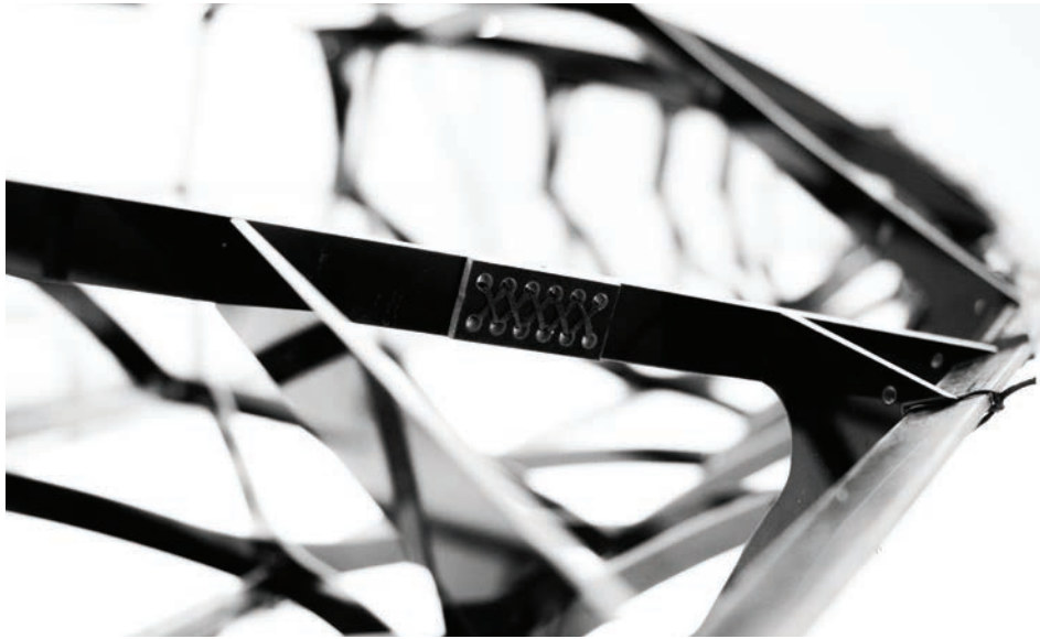
Figure 3.47 Polycarbonate Kayak. Revised mending plate connecting the seam of the ribs that facilitate the intersections.
