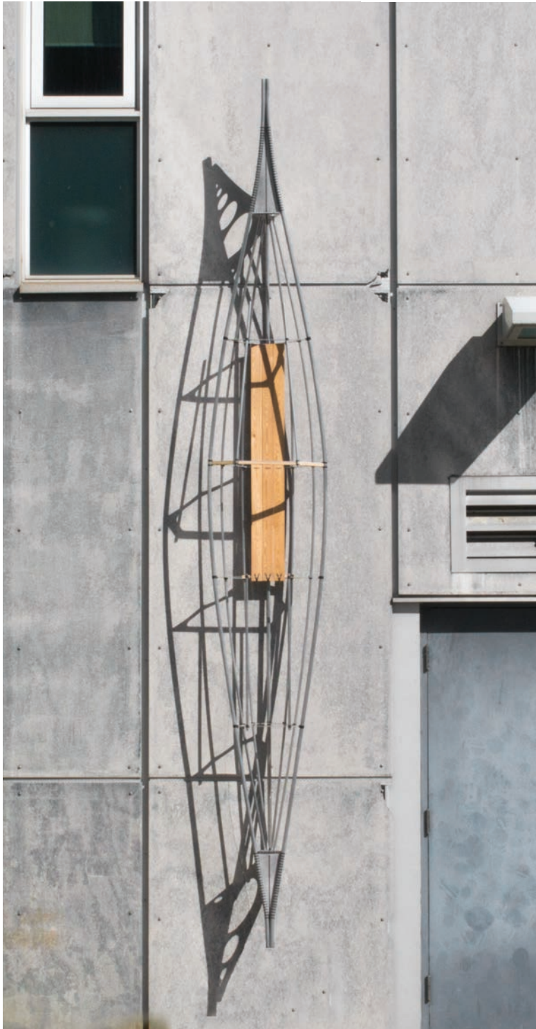
Figure 2.01 Aluminum frame kayak. Skin-frame-kayak resting against the architecture school facade.
