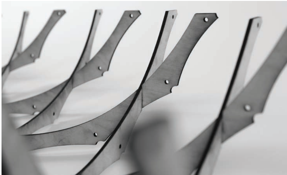
Figure 3.22 Attempt 2 of Isogrid Structure. Detail image of the intersection of the ribs with grooves cut for tubular rails.
