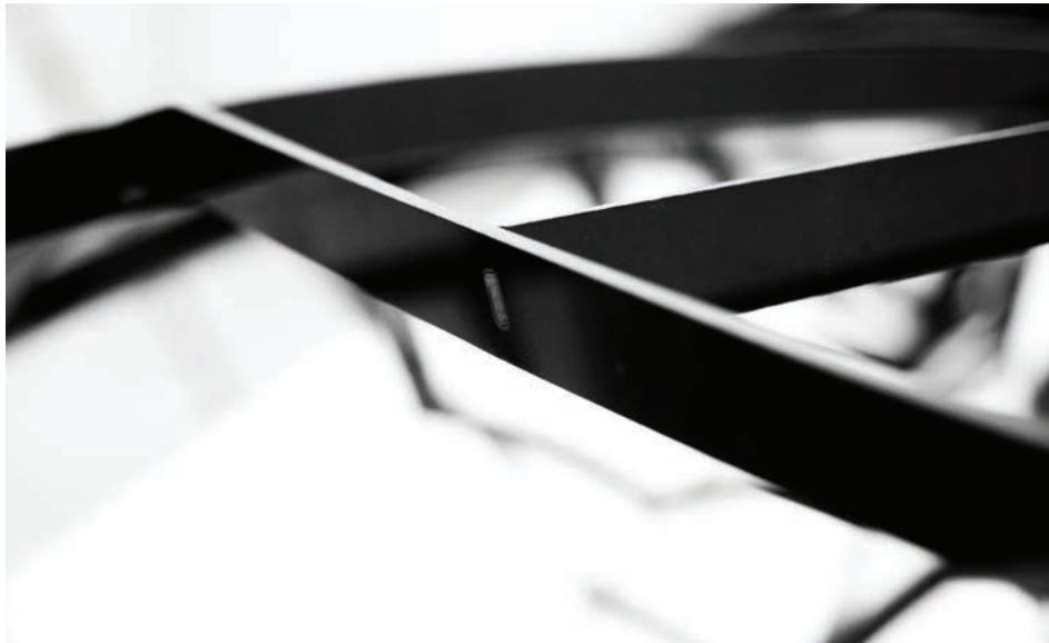
Figure 3.51 Polycarbonate Kayak. Photograph showcasing a mortise and tenon joint where two sets of ribs end to accommodate for a cockpit.
