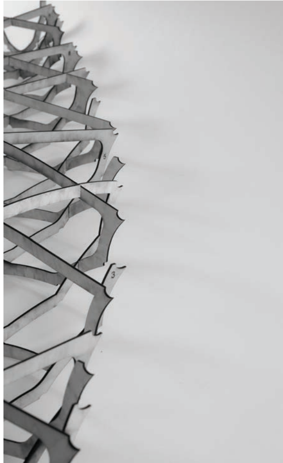
Figure 3.27 Attempt 2 of Isogrid Structure. The introduction of a closed isogrid slot rib intersections.
