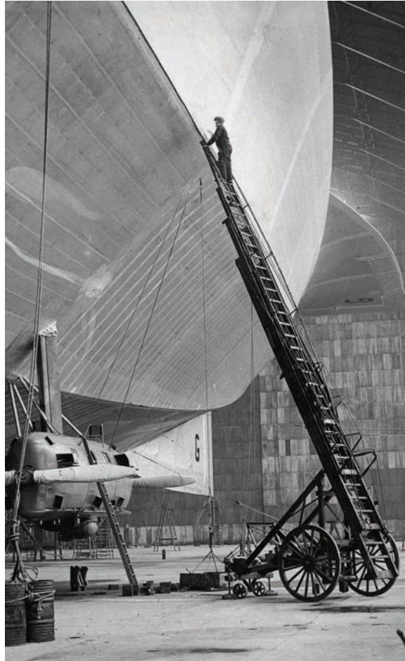
Figure 3.18 British Airship. The Barnes Wallis designed R-100 airship nears completion in its hangar in Yorkshire.
