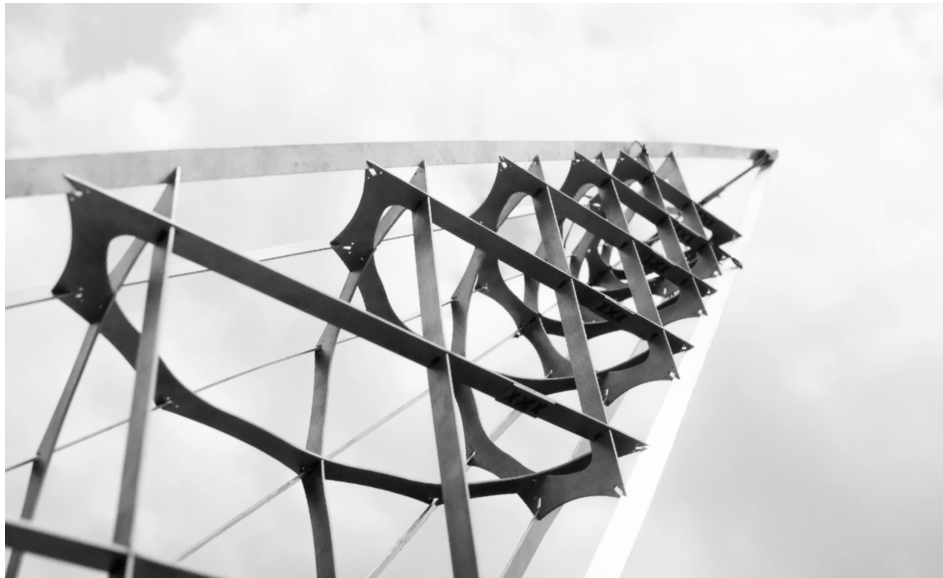
Figure 3.32 Attempt 3 of Isogrid Structure. View of the stern assembly of aluminum frame half scale model of geodesic isogrid kayak.
