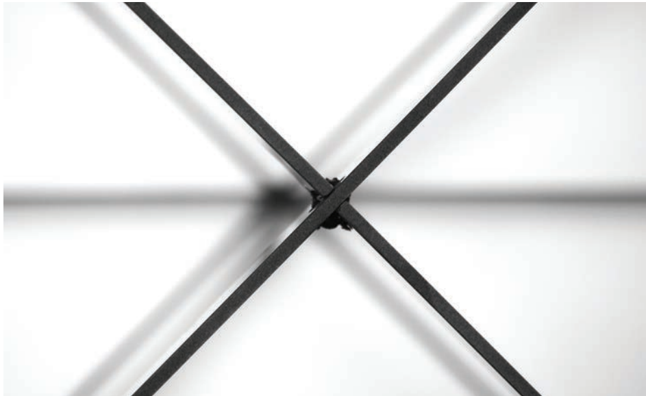
Figure 3.50 Polycarbonate Frame. Photograph of a slot joint and its lashing.
